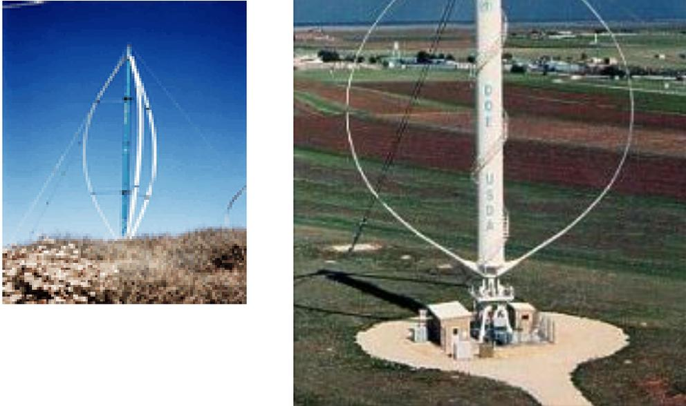
**FIGURE D-3 Examples of VAWTs (Left: FloWind Corporation VAWT at Tehachapi, California. Photo credit: R. Thresher. Source: Photo #04688, NREL 2004b. Right: Darrieus-design VAWT operated as a wind energy technology test bed by Sandia National Laboratories at the U.S. Department of Agriculture research station at Bushland, Texas; 138 ft (42 m) high, 112 ft (34 m) in diameter. Photo credit: Sandia National Laboratories. Source: Photo #01671, NREL 2004b.)**
