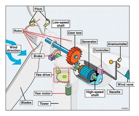
Anemometer: Measures the wind speed and transmits wind speed data to the controller.
